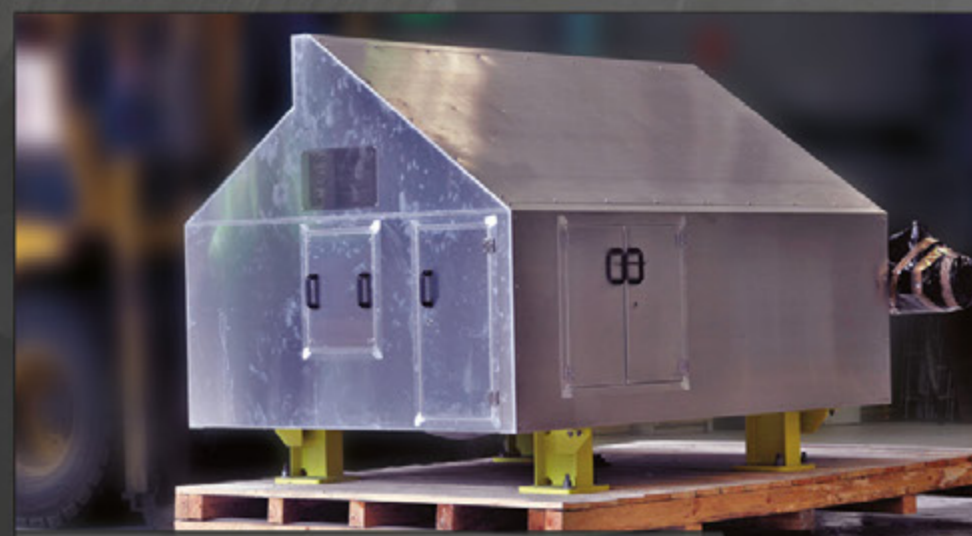
Winch covers in stainless steel designed for ease of maintenance
