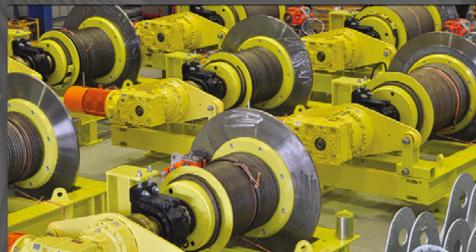
Take-up Winches - Western Turner Brockman Project, Hamersley Iron Pty Ltd.
